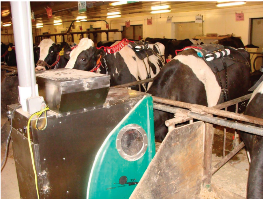
FIGURE 3.2 Simultaneous measurement of enteric methane emissions from dairy cows using the GreenFeed ® system (C-Lock Inc., Rapid City, South Dakota) and the SF_6 technique (courtesy of A. N. Hristov, The Pennsylvania State University).
