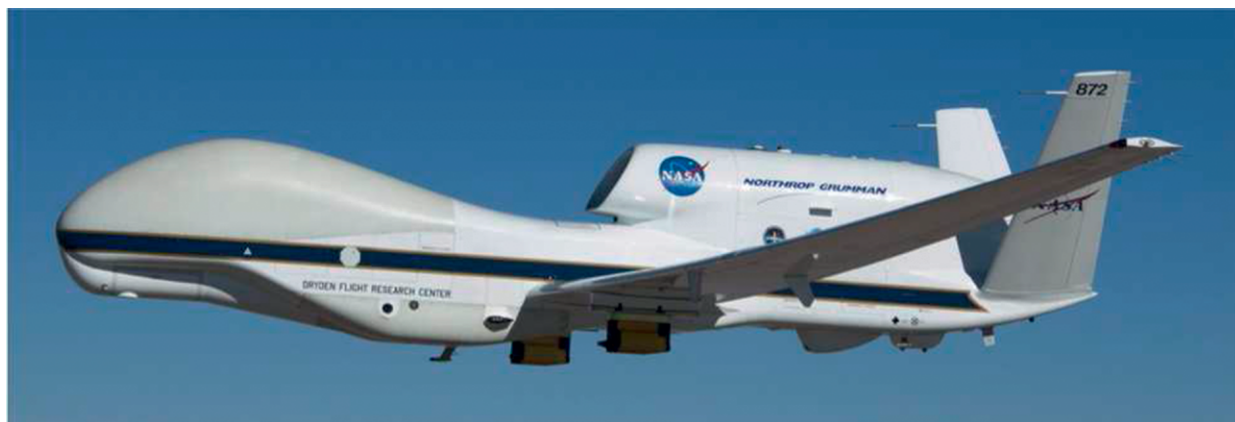
FIG. 2. The Global Hawk unmanned aircraft system. The wing pods, one with the Hawkeye instrument and the other with an aerodynamic/weight dummy for balance, are visible.
