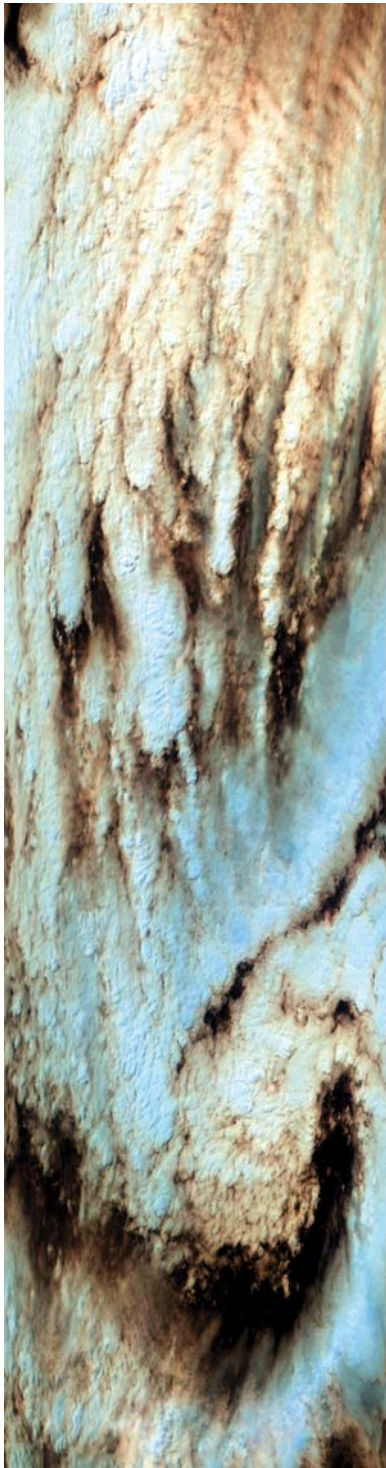
Figure 21. A false color MODIS-Aster Airborne Simulator (MASTER) image of the Von Kármán vortex sampled by the DC-8 on August 6 2007 just north of the Galapagos Islands (RGB = 2.1, 1.6, and 0.66 \mu\text{m} channels). The light blue color indicates relatively large cloud droplet sizes in these stratus clouds. The instrument's swath width (vertical dimension) is about 37 km, while the length of the flight leg is about 90 km. Image courtesy of Steven Platnick.
