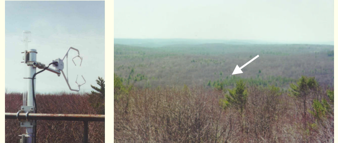
Figure 2. Left: Inlet and sonic anemometer at a height of 22m. The canopy height averages 20 m. Right: View of Harvard Forest with sampling tower location marked.
